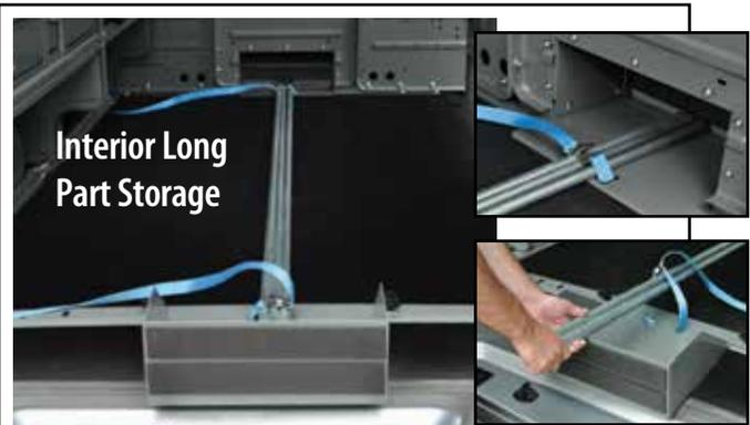
**Carry 10 feet of conduit or pipe inside your NV Cargo with the Long Part Storage Kit!**
