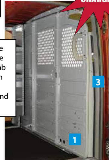
A cargo partition inside keeps your cargo in the back and helps with cab climate control. Bolt on partition accessories allow for easy access and organization.
