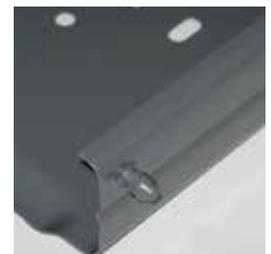
**Truly Adjustable Shelves** All you need is a phillips screwdriver! Simply remove two bolts from the speed nut clips that come with the shelf, tilt the shelf upwards, move the shelf to your desired location, insert the rear shelf studs, reattach the bolts and you're done!
