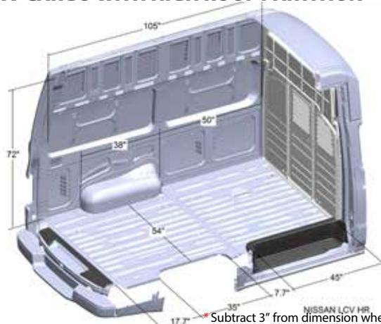
\* Subtract 3" from dimension when a Max Comfort partition wing kit is installed.
