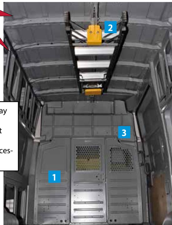
Keep ladders out of the elements and out of the way with an interior ladder rack. Store up to a 6 ft. step ladder inside your high roof NV Cargo. A full height cargo partition keeps your cargo in the back and helps with cab climate control. Bolt on partition accessories allow for easy access and organization.
