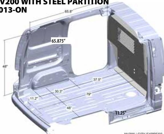
\* Measures 79" at the floor and up to 13" off the floor. Measures 72" at 23" and higher off the floor.
